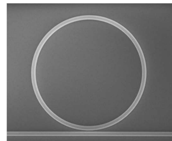
Figure 1: A single ring resonator coupled to bus waveguide
